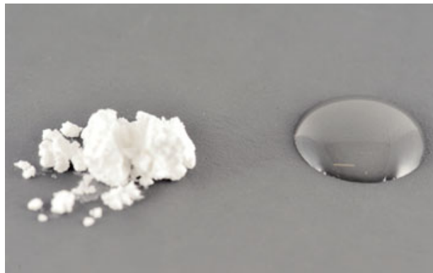
Fig 2 Example of fillers that are incorporated by mixing in a monomer mixture, thus producing a dispersed filler composite material.
