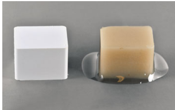
Fig 1 PICNs differ significantly from classic composite materials with dispersed fillers incorporated by mixing in a monomer mixture, in that a PICN material is the result of the infiltration of a pre-sintered glass-ceramic scaffold with a monomer that is secondarily polymerized. This ceramic network forms a real skeleton, with specific mechanical properties.
