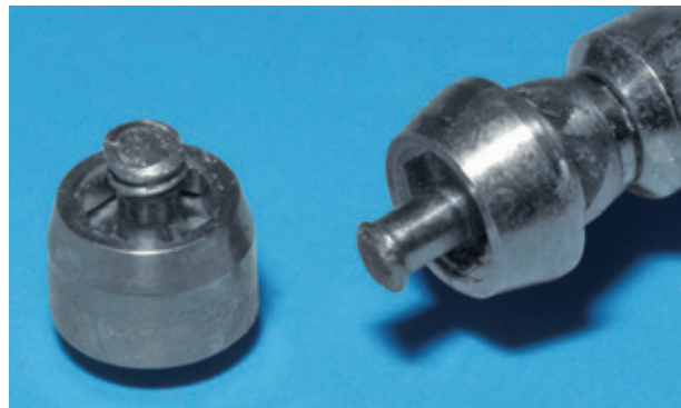
Fig 1b The broken titanium screws with the respective transmucosal abutments.
